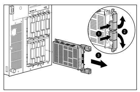
Figure 2-19. Removing a Wide-Ultra hot-plug hard drive
